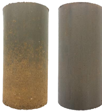
Fig. 5. Insufficient Compaction (Left), Uniform Compaction (Right)
