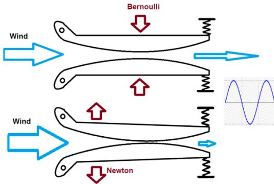
The aerofoils are hinged and sprung and wind passing over the curved surfaces results in lift (Bernoulli) forcing the aerofoils to close in on themselves. At a certain point the air speed drops and wind momentum change forces the aerofoils apart (drag, Newton). This creates an oscillating motion of a few centimetres whose energy can be used for power generation. To convert this we use a combination of tribo-electric charge generation and variable capacitance electrical voltage generation.
