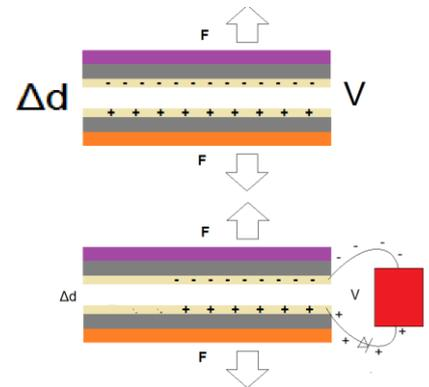
the standing voltage of the storage cell to complement the capacitive voltage  $V_1$  and create  $V_2$  which is greater than  $V_1$ . As this cycle repeats the voltage stored on the cell grows as a function of the work done. The storage cell energy is then used to charge a battery system, which later feeds the grid. Please reference our patent application GB1620410.9 for full details.
