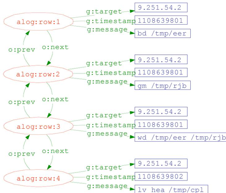
Figure 5: The log described in Table 2 after transformation into RDF.
