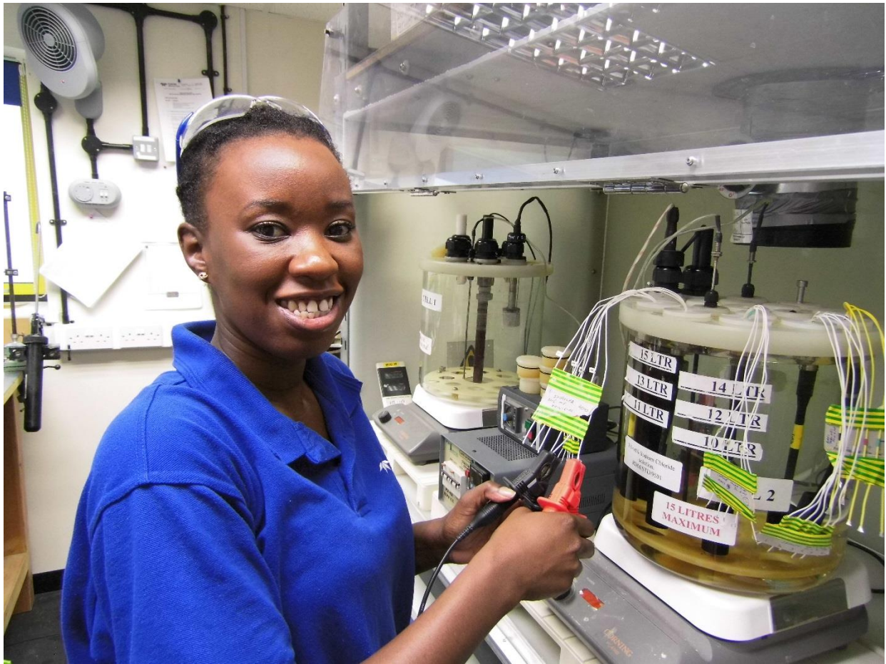
Jamila Joseph carrying out electrochemical measurements on a test cell in the Dr Sheelagh Campbell Laboratory.
