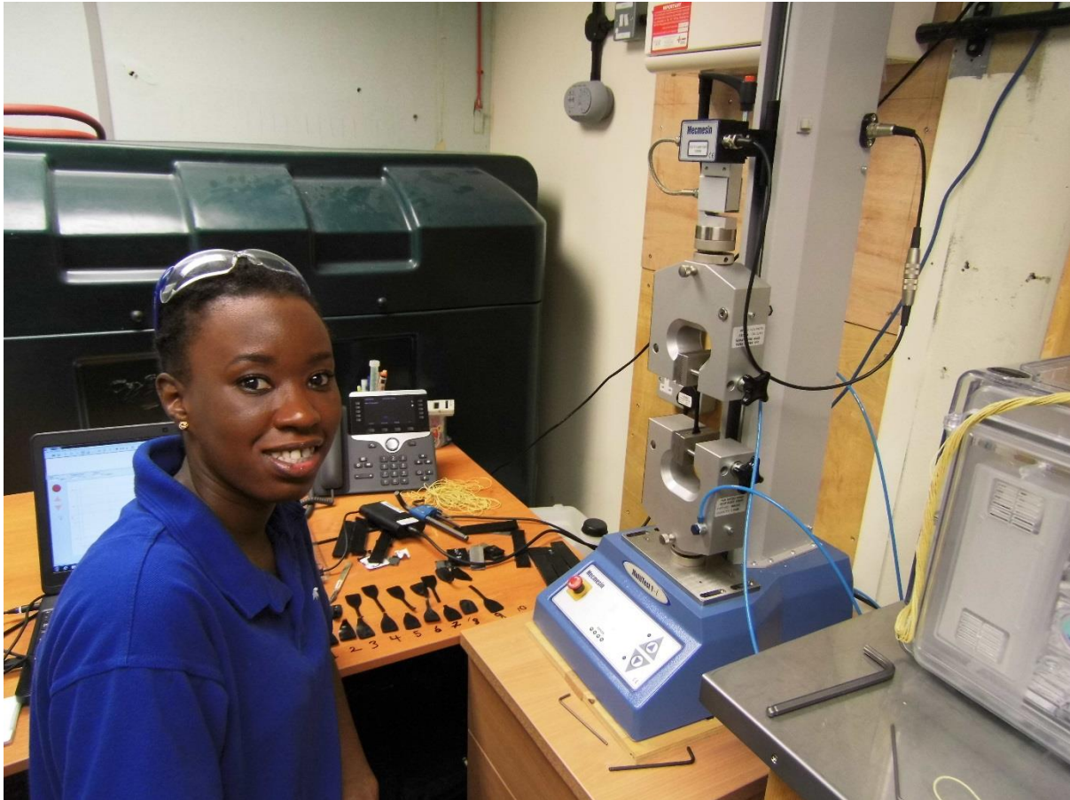
Jamila Joseph, in the Dr Sheelagh Campbell Laboratory, carrying out tensile strength measurements of PU test pieces. The same equipment is used, with minor modification, for measuring PU-metal adhesion bond strengths (pull-tests).
