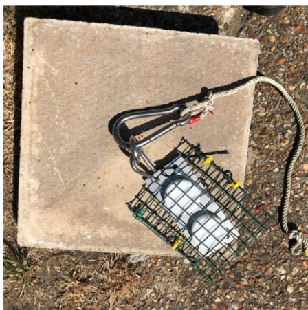
Fig. 7. Stainless steel plate attached to the deployment concrete slab and deployment rope attached to eye bolt.
