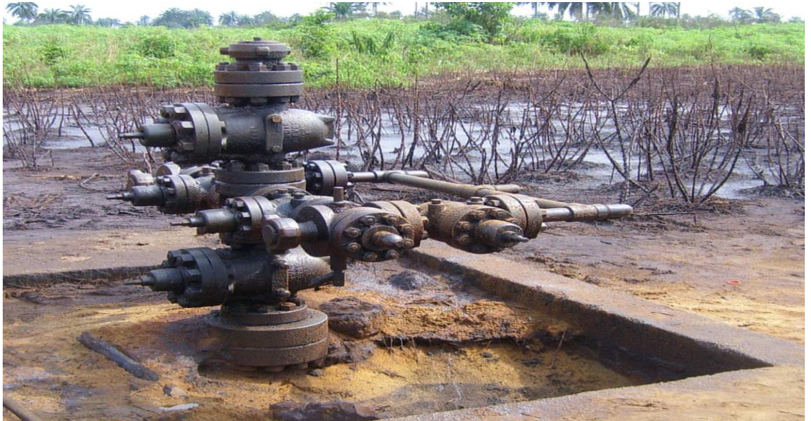
Figure 2.5: Typical blown-out wellhead in the oil-producing Niger Delta region, Nigeria (Okop, 2010)
