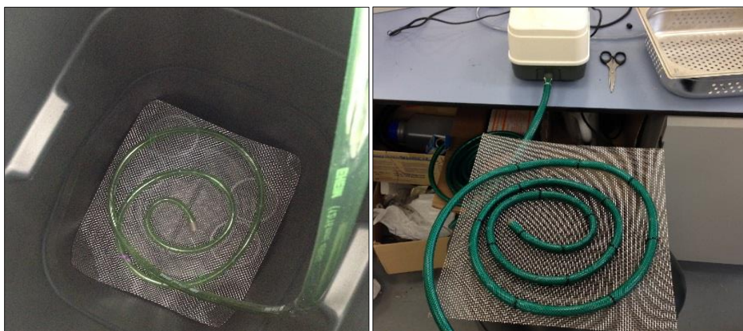
Figure 3.8: Perforated tubing for air supply.
