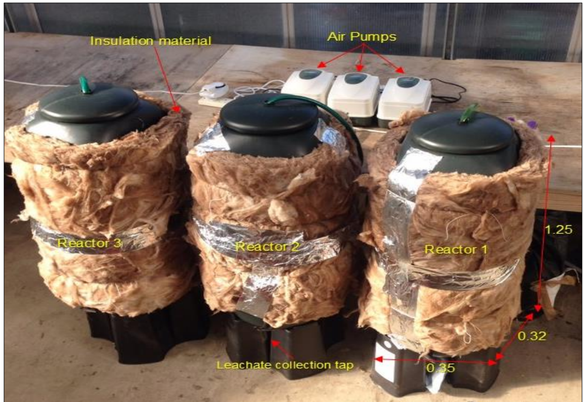
Figure 3.7: Experimental set-up of the mesocosm test showing the external air supply and reactors wrapped with the insulation material.
