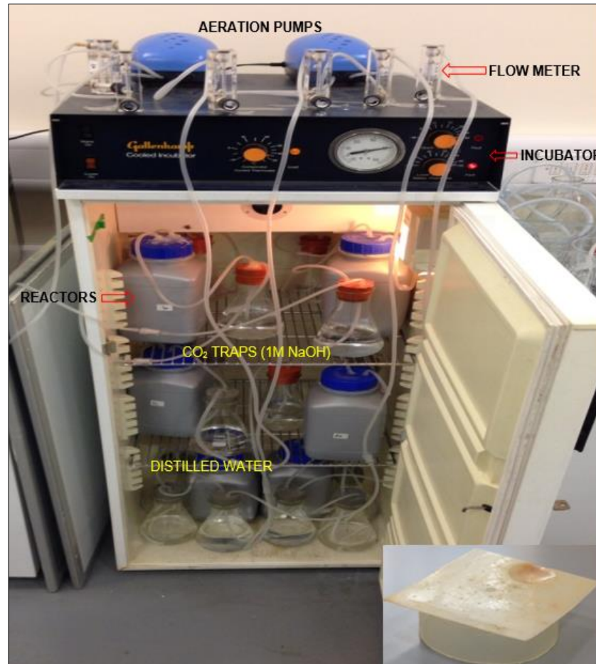
Figure 3.4: Experimental set-up of the microcosm experiment showing the incubator and aeration system. The image inset shows the rectangular perforated plastic floor supported by a semi-rigid ring on which sample mix is placed within the reactor vessel.
