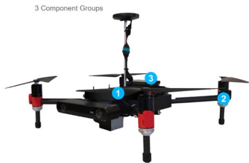
Figure 4 Overview of AIR 4 LIGHT, 1-body, 2-detachable arms, 3-battery
