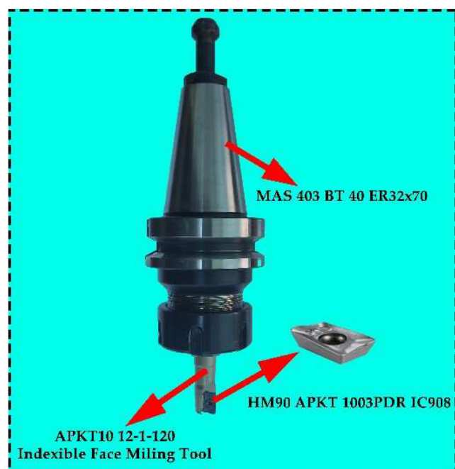
Fig. 1 – Cutting tool clamping system.
