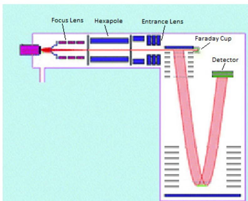
Figure 1.11 Schematic representation of the lens system of a time of flight mass spectrometer (Tong, Yu, Jin, Hi, Hang and Huang, 2009)
