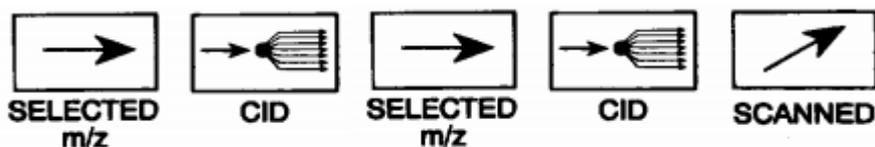
Figure 1.20 Diagrammatic representation of an  $MS^3$  scan (adapted from de Hoffman, 1996)
