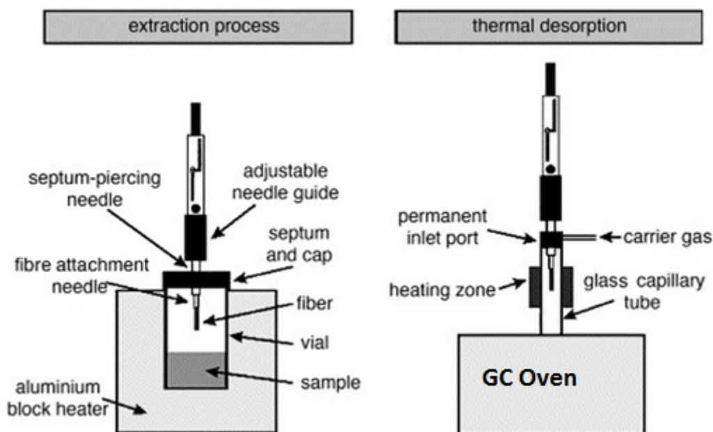
Figure 1.2 Diagram of solid phase microextraction with thermal desorption (Barié, Bücking and Rapp, 2006)
