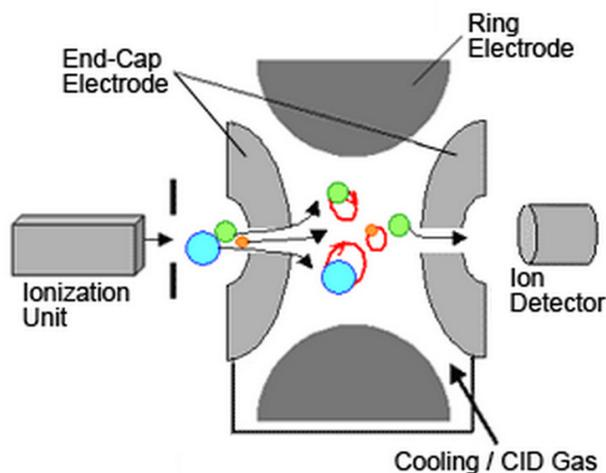
Figure 1.9 Sectional view of a quadrupole ion trap to show the similarity to a quadrupole (Shimadzu, 2014)
