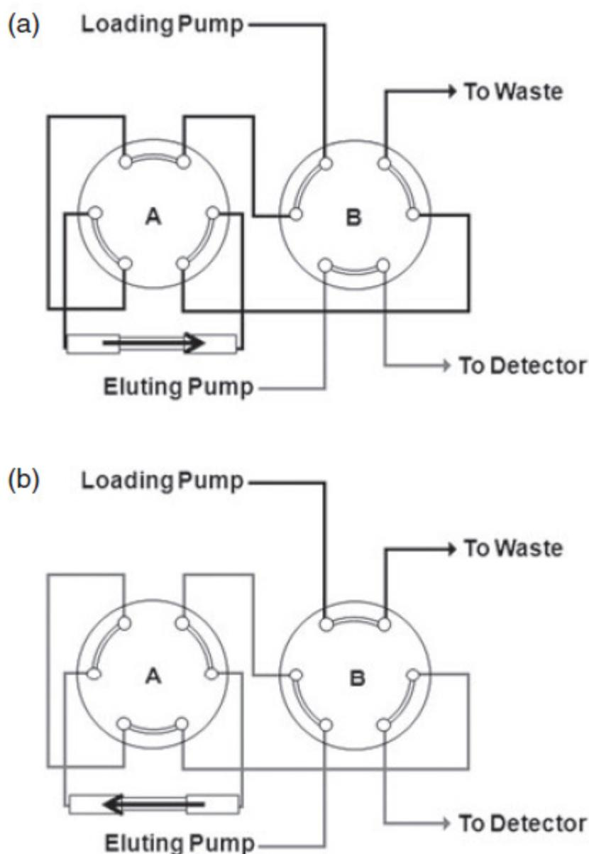
Figure 1.3 Plumbing of a Turboflow<sup>®</sup> System showing the valve arrangement (Couchman, 2012)
