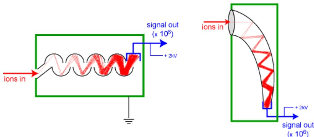
**Figure 1.15 Comparison of the structures of discrete and continuous dynode electron multipliers (Gates, 2004)**
