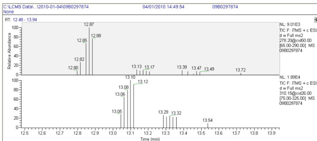
**Figure 3.6** Chromatogram demonstrating the effect of poor Dynamic Exclusion settings (Upper trace: EDDP, lower trace: Methadone)
