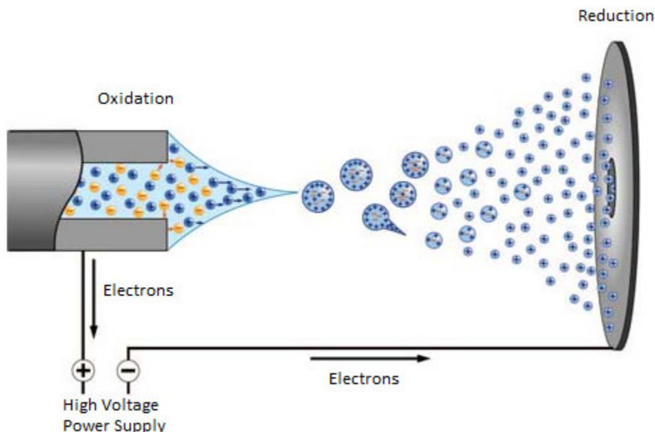
Figure 1.14 Image of an electrospray ionisation source showing coulomb explosion (Dahlin, 2008)
