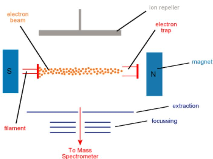
Figure 1.13 Schematic representation of an electron ionisation source (Gates, 2005)
