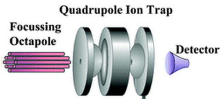
Figure 1.8 Schematic arrangement of the lenses of a quadrupole (3D) ion trap (O'Hair, 2006)
