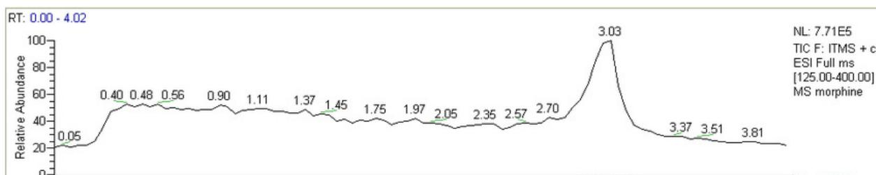
Figure 3.5 Optimisation of Turboflow® Cyclone MAX column retention: morphine retained on Turboflow® column for 3.03 minutes, demonstrating excessive retention
