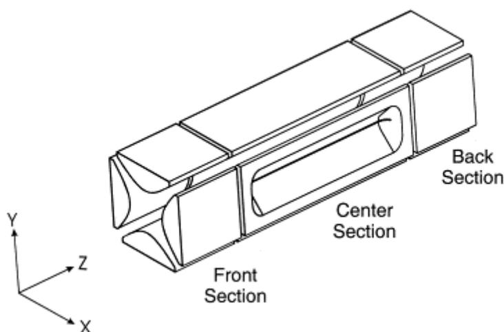
**Figure 1.10** Diagram of a linear (2D) ion trap showing the ion exit slit in the centre section (Shwartz, Senko and Syka, 2002)
