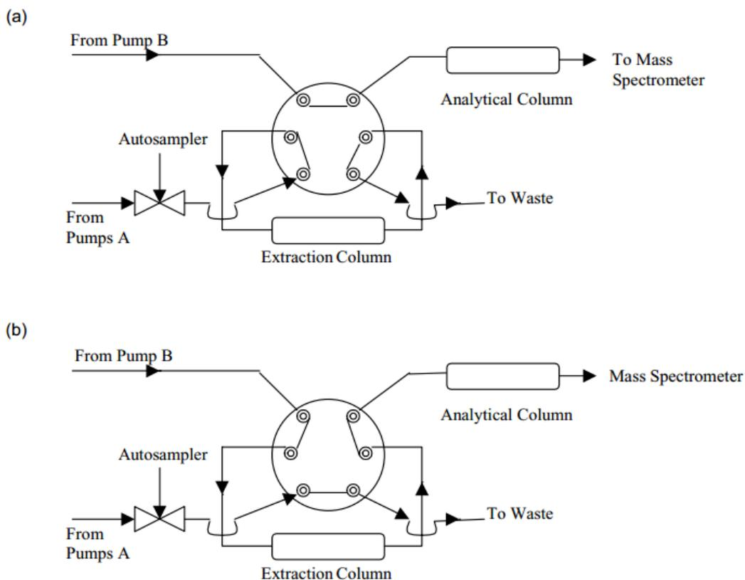
**Figure 1.1** Plumbing arrangement of an online SPE system using 6-port valve (Xu, Turner, Meeker, Pursley, Arnold and Unger, 2003). a) Sample loading step with analytical column bypassed, b) Sample elution step. After sample elution, the valve is reset to position a) for extraction column regeneration
