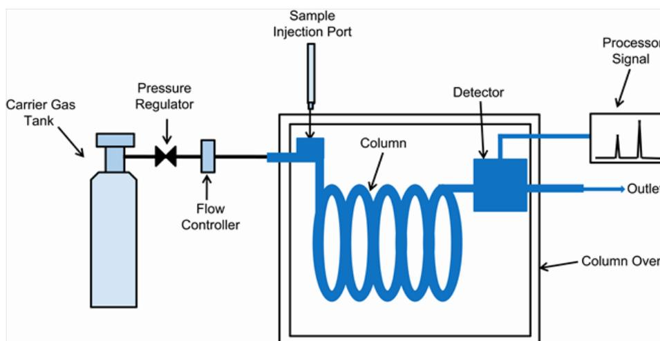
**Figure 1.4 Schematic diagram of the main components of a gas chromatography system (Philadelphia College of Pharmacy, 2012)**
