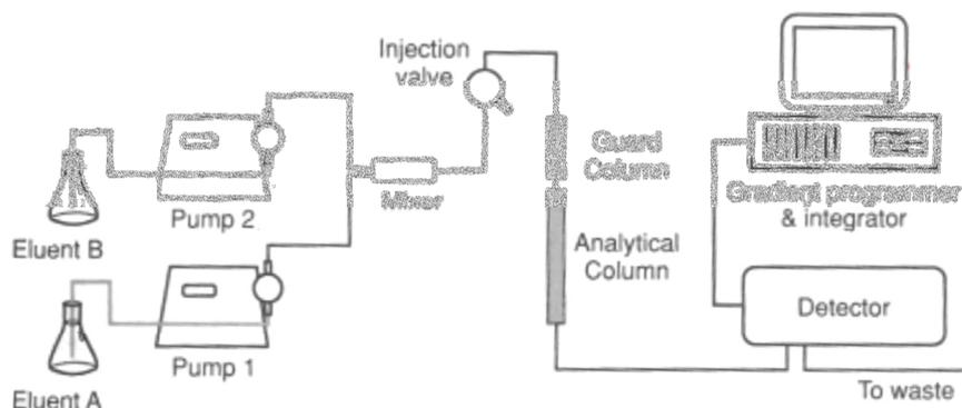
**Figure 1.5** Diagram of the main components of a typical HPLC system (Flanagan, Taylor, Watson and Whelpton, 2007, p. 179)
