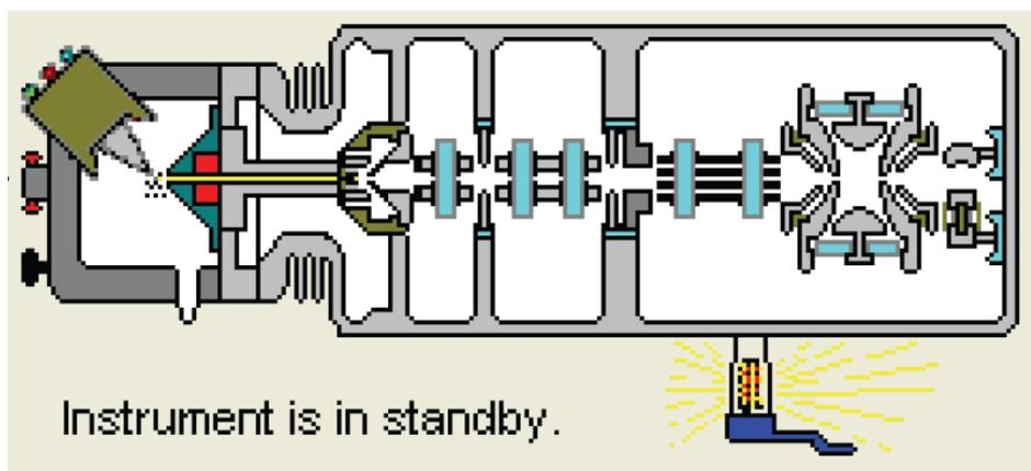
Figure 2.1 Schematic arrangement of the LCQ Fleet ion optics (Xcalibur screenshot)
