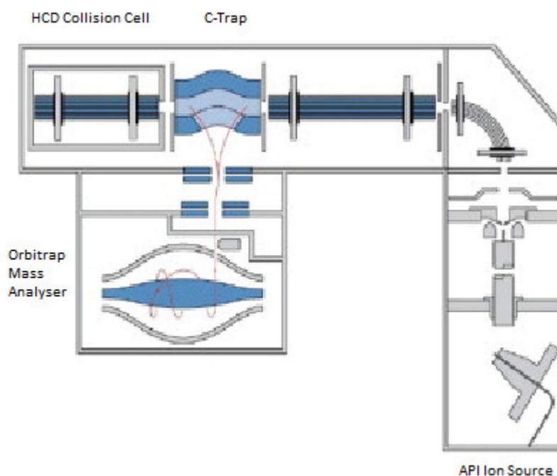
**Figure 1.12** Diagrammatic representation of the lens system of an orbitrap mass spectrometer (Bateman, Kellman, Muenster, Papp and Taylor, 2009)
