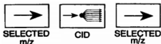
Figure 1.18 Diagrammatic representation of selected reaction monitoring (adapted from de Hoffman, 1996)
