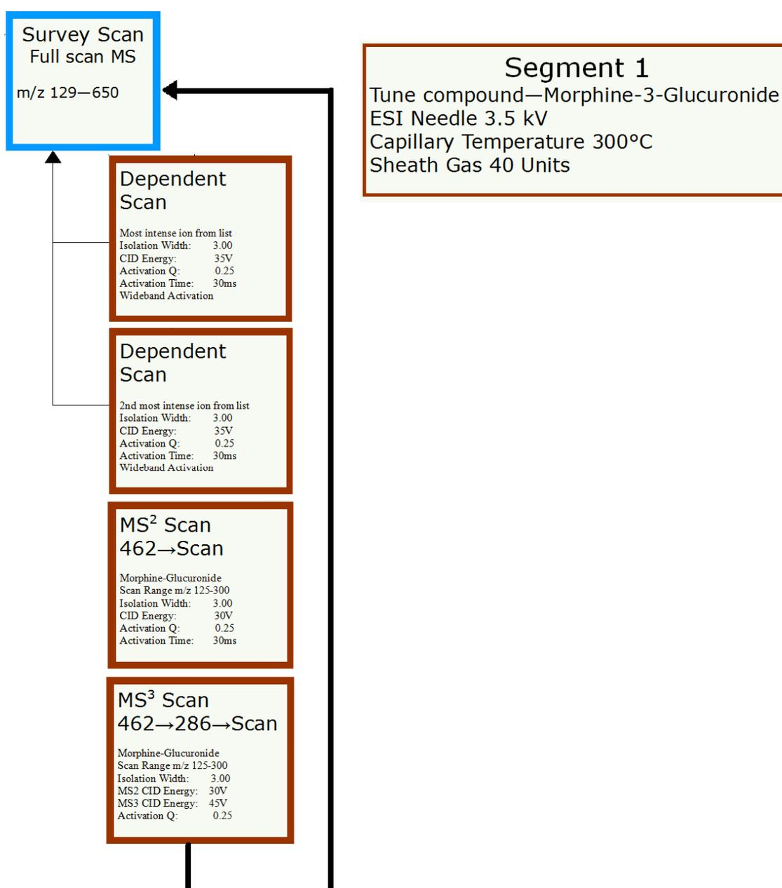
Figure 3.1 SPE Method Segment 1 scan parameters
