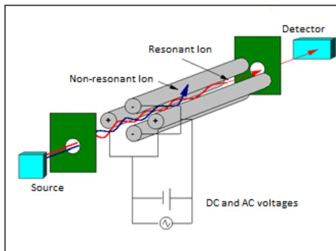
**Figure 1.7 Schematic arrangement of a quadrupole mass spectrometer lens system (Tissue, 2000)**
