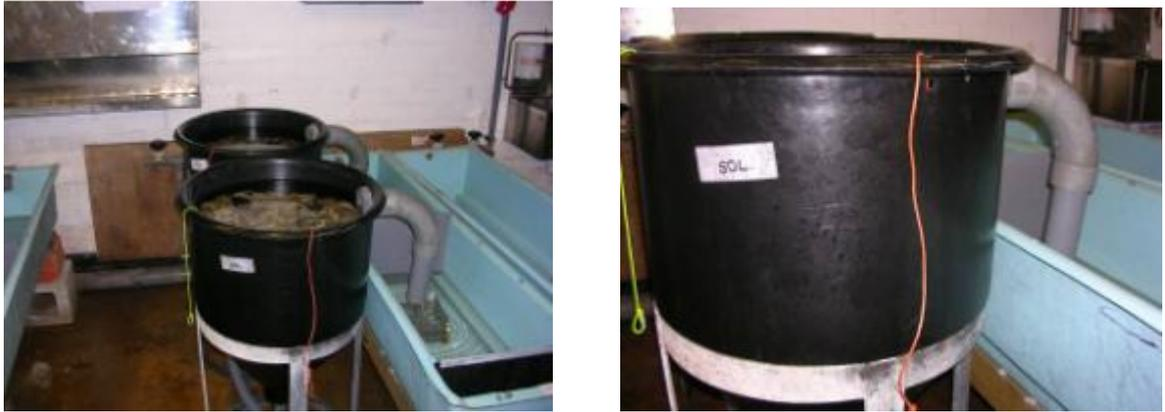
**Figure 5.3. Incubators used for sediment trials i) showing emergence tank; ii) incubator.**
