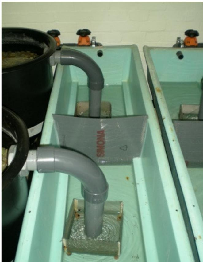
**Figure 5.2. Emergence tanks showing mesh box to catch the swim up fry.**
