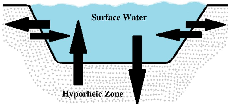
**Figure 1.5. A schematic of the hyporheic zone. The arrows indicate the movement of water between the surface water and hyporheic zone. (Drawn by author).**
