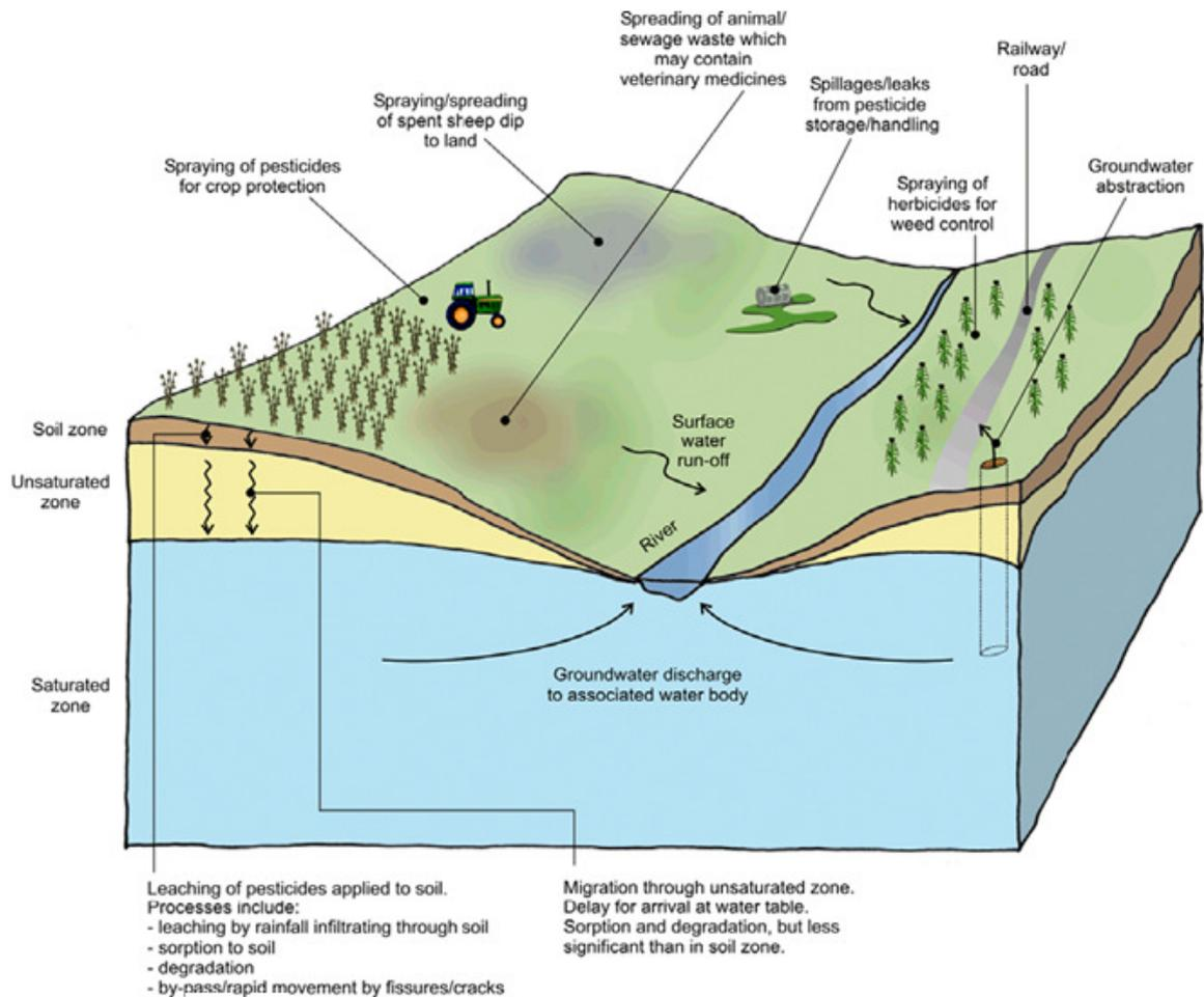
**Figure 1.6. Routes of entry into the freshwater environment (Pesticide sources, pathways and receptors, courtesy of EA).**
