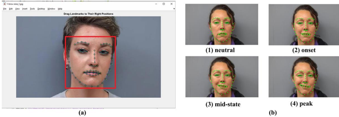
Fig. 3. Database annotations. (a): A screenshot of the software used to annotate facial landmarks. Only one detected face in each image is detected (shown in the red bounding box) and annotated (green circles) by the software. If some landmarks need to be adjusted, annotators drag those landmarks (black circles) directly to their right positions manually. (b): Sample face of four keyframes (1) neutral, 2) onset, 3) a mid-state between onset and peak, 4) peak) with 68 landmarks automatically annotated using the Supervised Descent Method (SDM) [39] method and manually corrected by our annotators.
