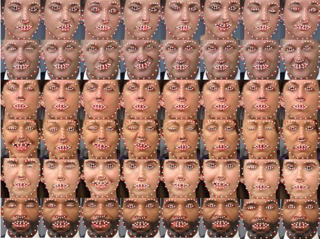
Fig. 6. Example results in each row are detection results of facial landmarks for the samples in the AFLFP database, where 68 landmarks were employed for evaluation. Red: ground truth from. White: predictions of the proposed method.
