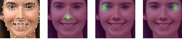
Fig. 5. The sample heatmaps generated using Gaussian kernel. The first left image shows the ground truth facial landmarks. The others show some sample generated heatmaps of facial landmarks (with the original image behind). From left to right: nose ridge tip, right eye corner outer and left eye corner outer.
