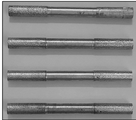
Figure 5. Casted samples machined into the tensile test specimen.
