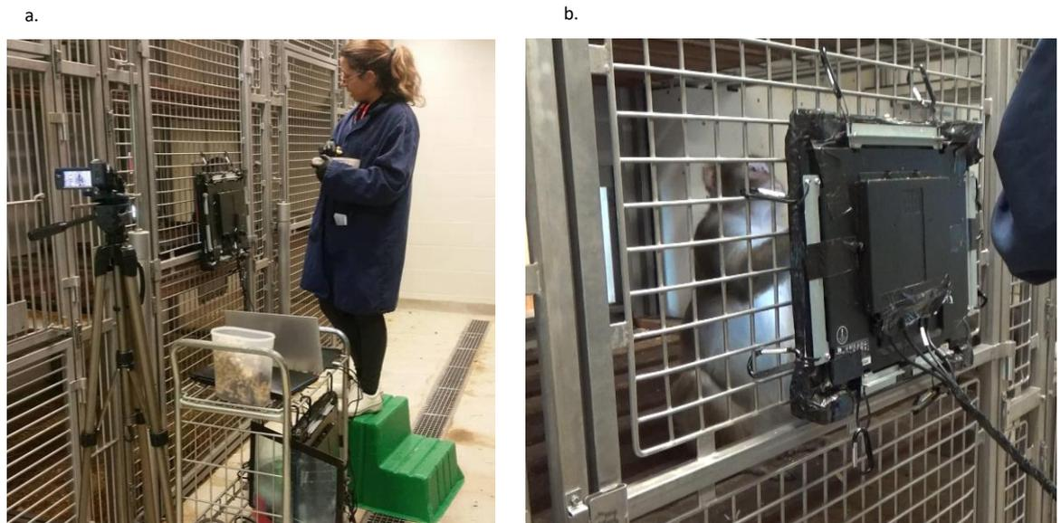
Figure 2.3. Apparatus used in the experiments. A laptop was connected to a touchscreen attached to the cage bars (a). Sessions were recorded thanks to a video camera. Individuals sat in front of the screen (b) and rewards (dry raisins for the tested individual) were given by hand.
