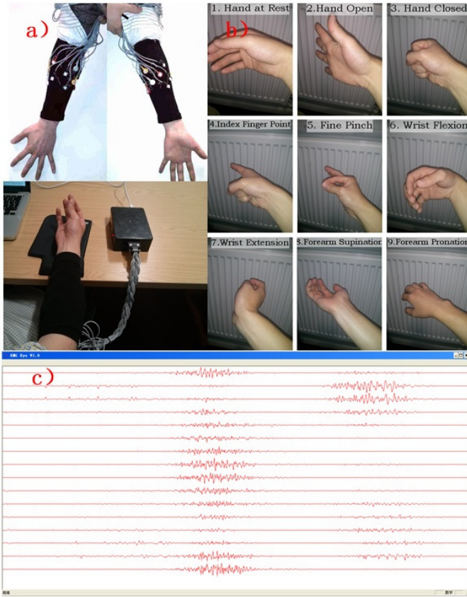
Fig. 4. From left to right, top to bottom: a. sEMG acquisition hardware including electrodes embedded sleeve and processing circuit b. 9 motions to be recognized c. display of 16 channels' sEMG samples [17]
