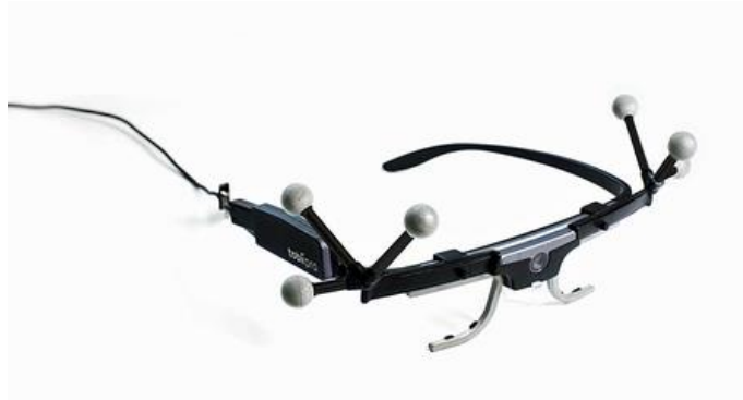
Figure 4.1: Tobii Pro glasses 2 with motion capture markers attached.
