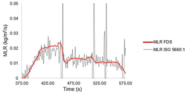
**Fig. 7** Cone calorimeter experimental MLR recordings (black lines) vs FDS predicted MLR (red line) (Color figure online)
