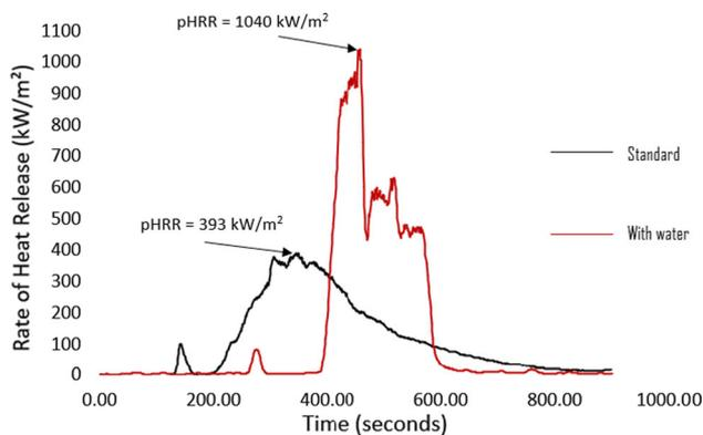
**Fig. 3** Cone calorimeter experimental heat release rate vs time, standard (black line) vs with water (red line) (Color figure online)
