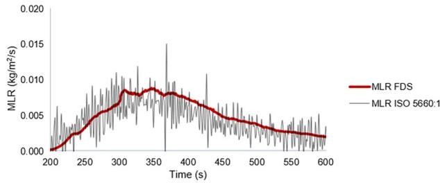
**Fig. 6** FDS predicted MLR (red line) vs cone calorimeter MLR recordings (black lines) (Color figure online)
