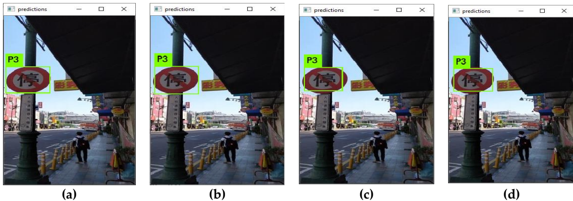
Fig. 13 Recognition result Class P3 employing (a) Yolo V4_1, (b) Yolo V4_2, (c) Yolo V4-tiny_1, (d) Yolo V4-tiny_2.
