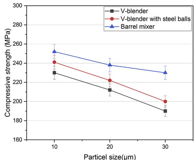
Fig. 9 – Impact of particle size on compressive strength of Al-MMC.
