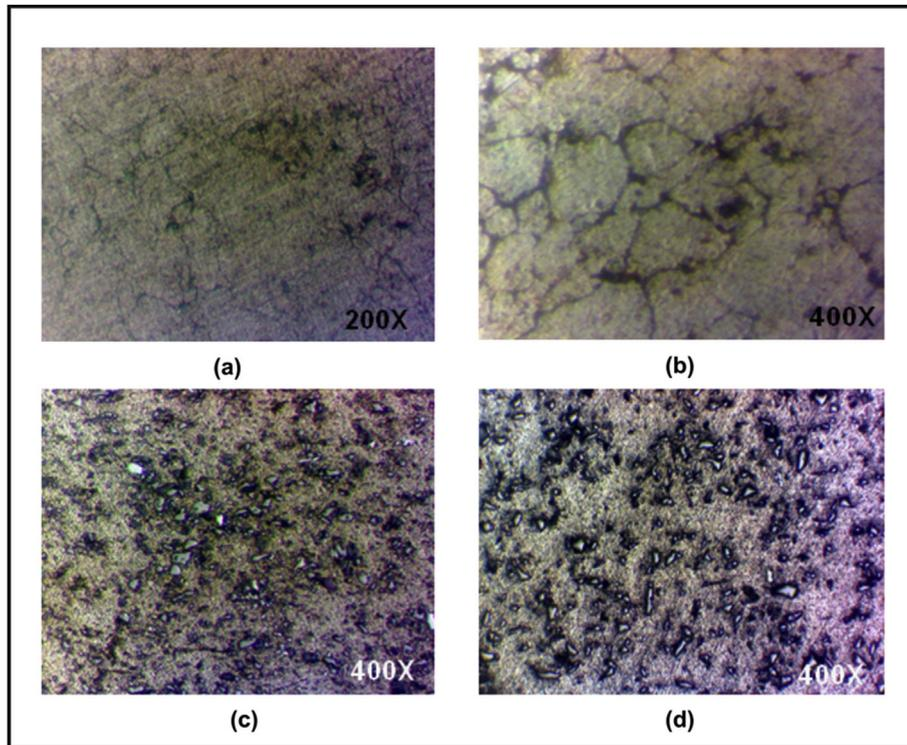
Fig. 3 – Optical images of Al-MMC (a) and (b) without reinforcement (c) 15% SiC and (d) 20% SiC mixed with barrel mixers.
