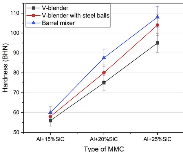
Fig. 7 – The hardness of Al-MMC with varying content of SiC and mixing methods.
