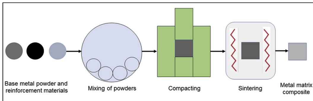
**Fig. 1 – Schematic illustration of the powder metallurgy technique to prepare MMCs.**
