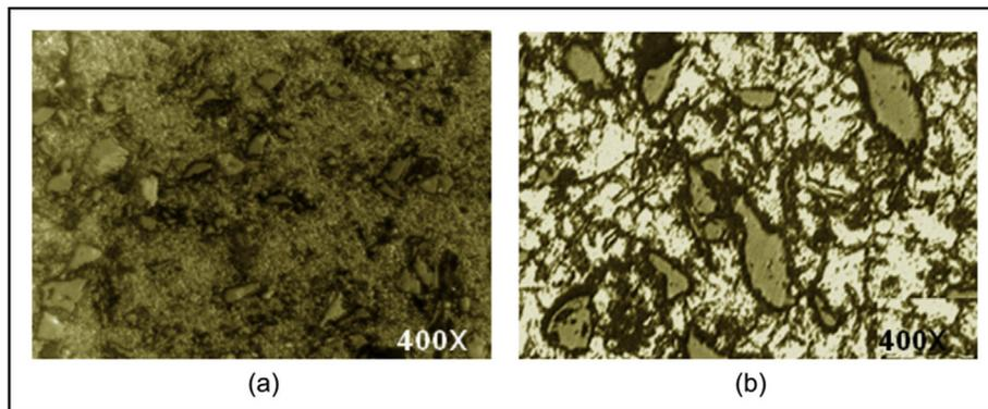
Fig. 4 – Microstructure of Al-MMC with (a) 15% SiC and (b) 20% SiC mixed with V-blender.
