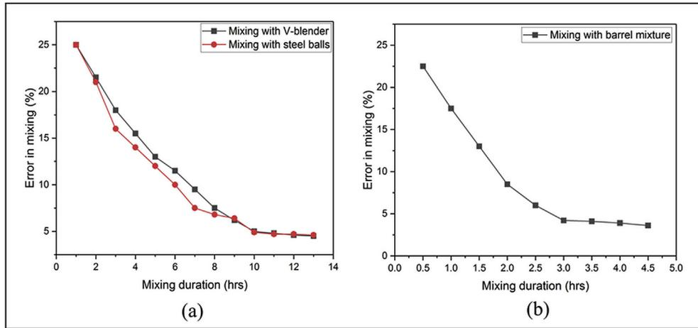
Fig. 6 – (a) Mixing of powders with v-blender (b) Mixing of powders with barrel mixer.
