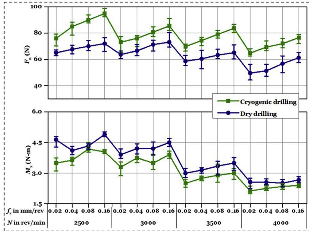
Fig. 4 – Variation in  $F_n$  and  $M_z$  using dry and cryogenic drilling.
