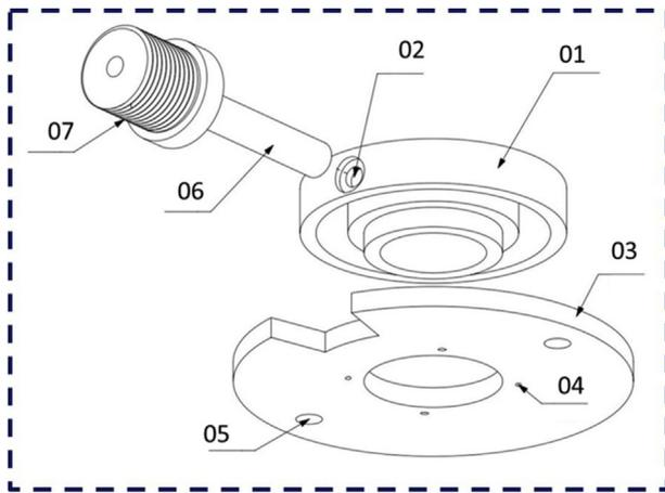
Fig. 3 – Multi-jet LN<sub>2</sub> delivery nozzle schematic.
