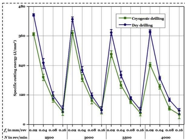
Fig. 5 – Variation in SCE using dry and cryogenic drilling.
