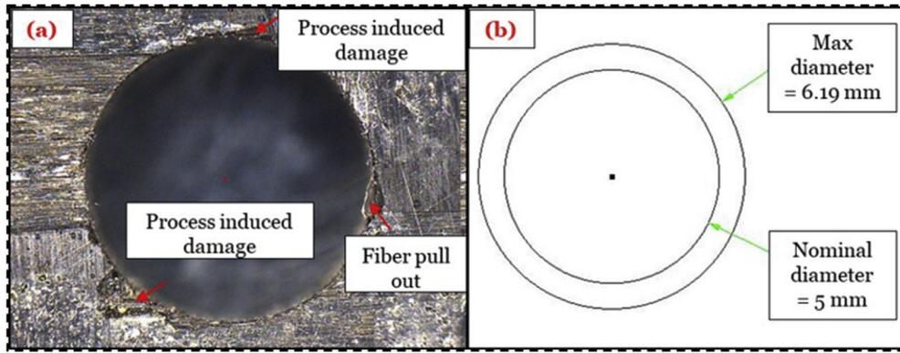
Fig. 6 – Damage measurement (a) image of a hole (b) maximum and nominal diameters calculation.
