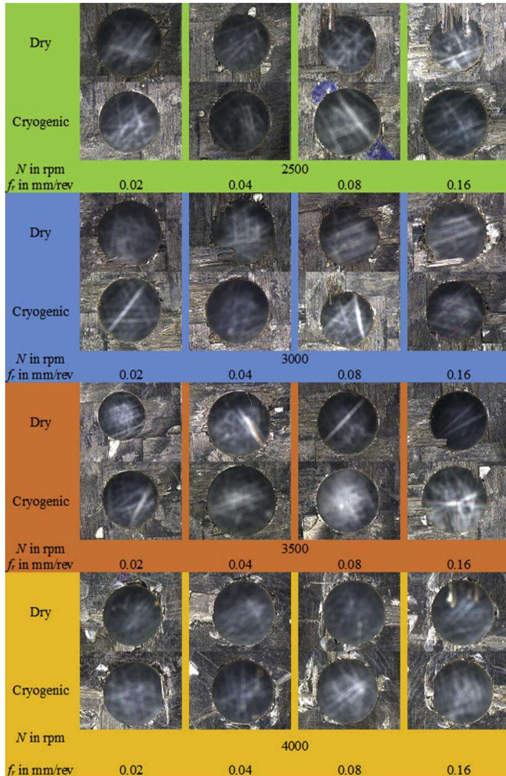
Fig. 9 – Observation of the entry surface at various combinations of  $N$ ,  $f_r$ , and cutting conditions.
