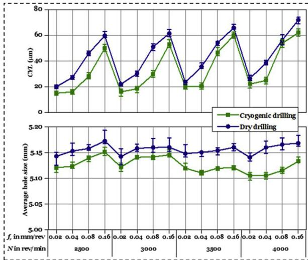
Fig. 10 – Variation in CYL and average hole size using dry and cryogenic drilling.
