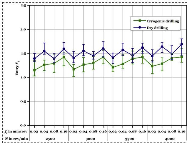
Fig. 7 – Variation in entry  $F_d$  using dry and cryogenic drilling.
