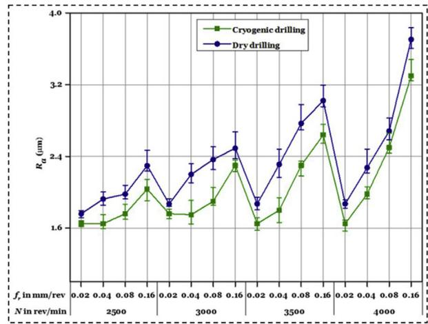
Fig. 11 – Variation in  $R_a$  using dry and cryogenic drilling.
