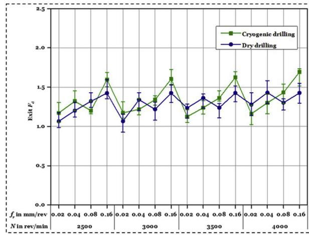
Fig. 8 – Variation in exit  $F_d$  using dry and cryogenic drilling.
