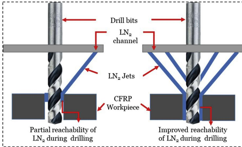
Fig. 1 – Schematic of an improved multi-jet LN<sub>2</sub> delivery system.
