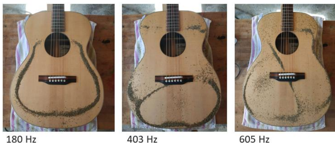
Fig. 11 Complete build of the instrument using the X-bracing pattern simulated here (see fig. 9)
