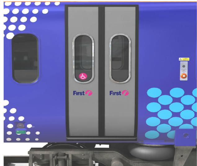
**Fig. 5** The Class 380 train's passenger door unit
