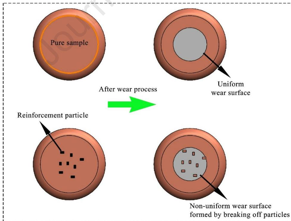
Fig. 13: Uniform surface formation after wear process
