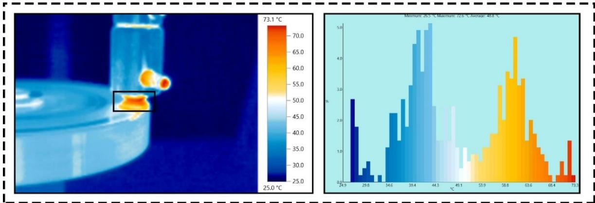
Fig. 3: Temperature distribution graph of the image taken during the wear test
