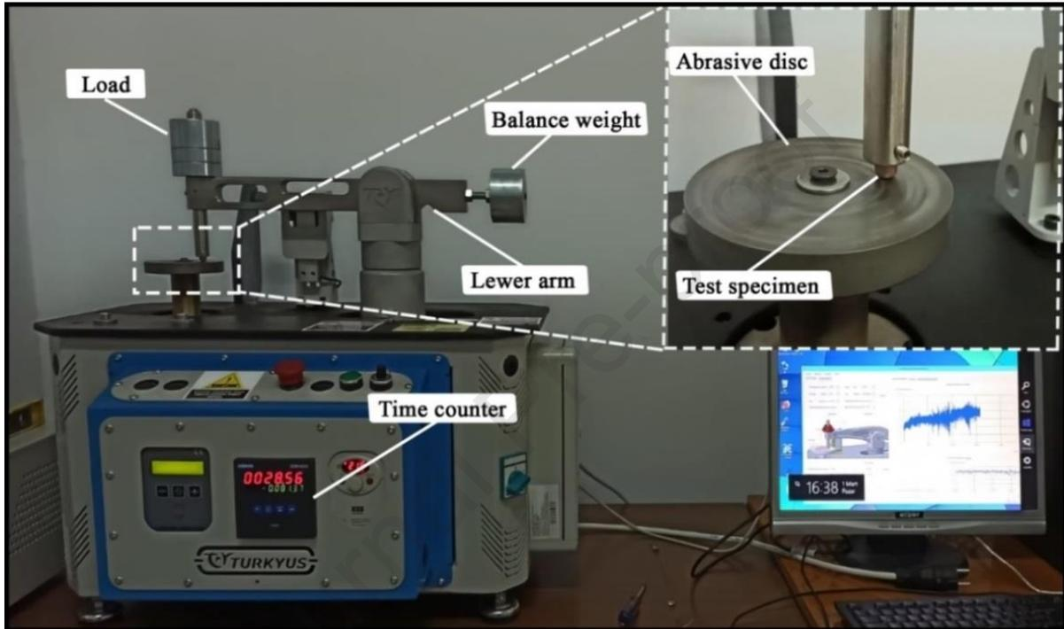
Fig. 2: Details of the wear device used in the analysis
