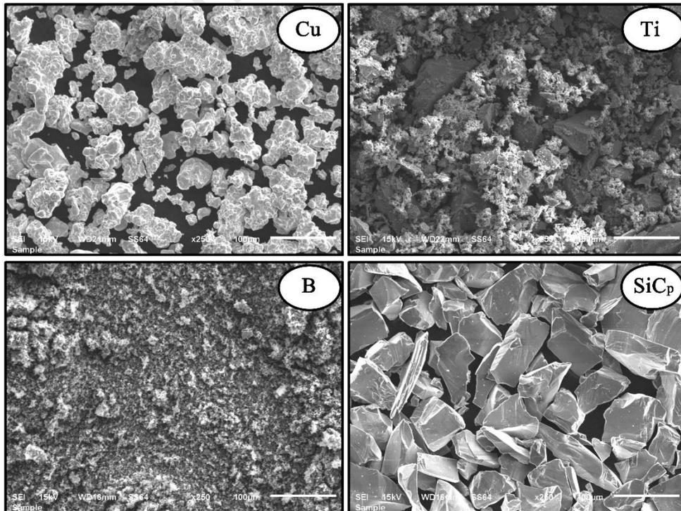
Fig. 1: SEM images of the powders used in the experiment [6, 22]
