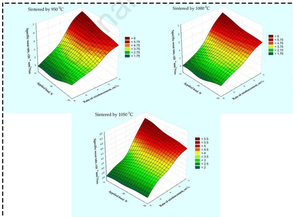
Fig. 9: SWR graph of produced composite materials
