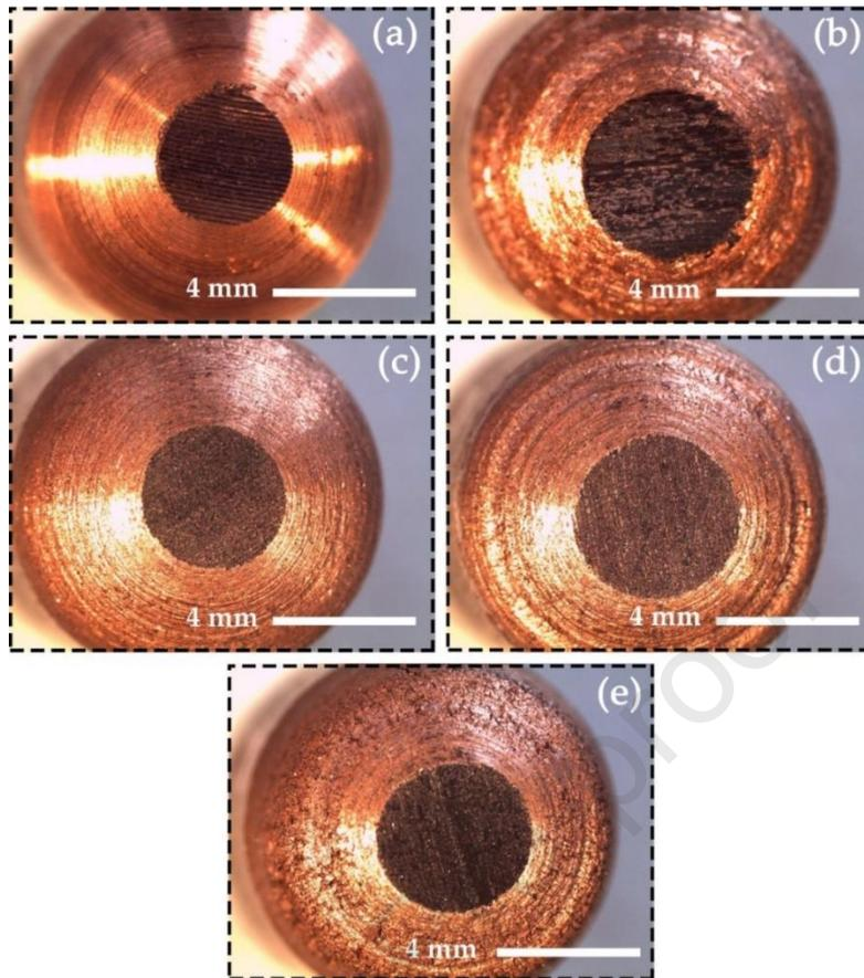
Fig. 12 Wear diameter photographs of composites produced in different proportions:
