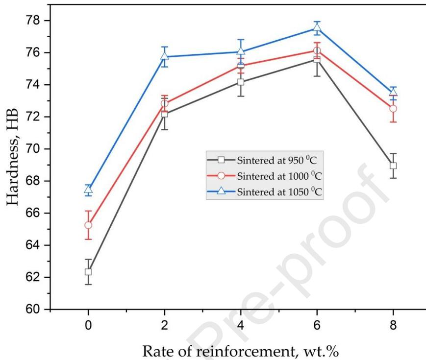
Fig. 8: Hardness graph of produced composite materials
