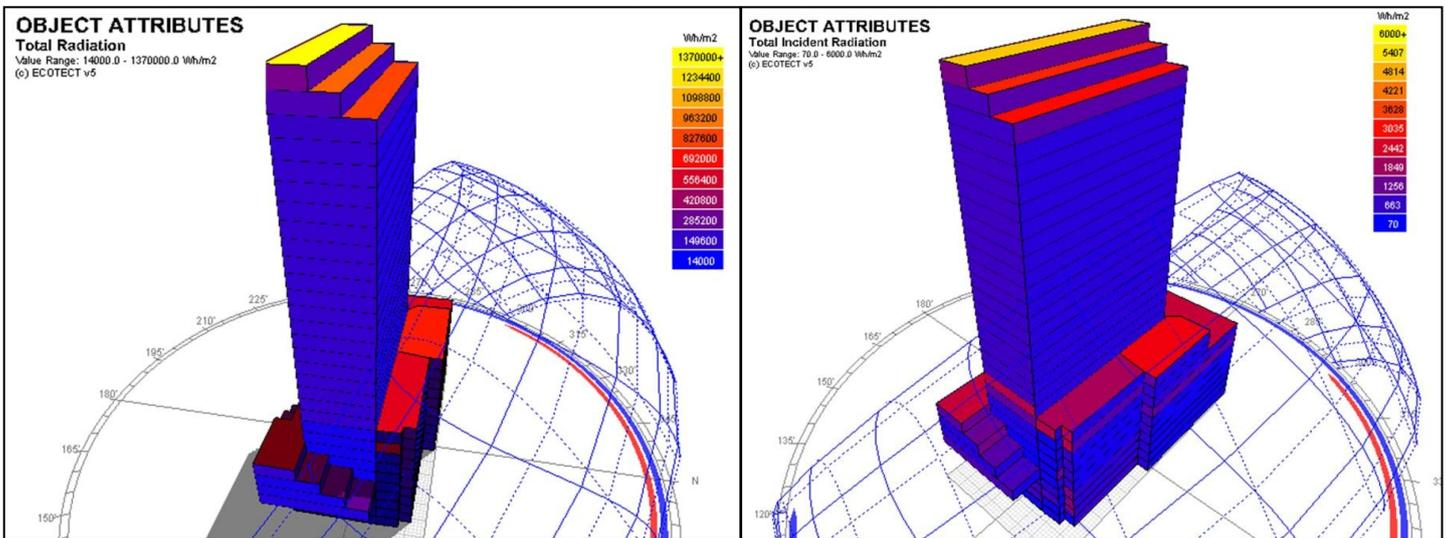
Total radiation absorption by **EXISTING BUILDING FABRIC**. note the range is between 14 to 1370 kwh/m<sup>2</sup>. Derived from: Autodesk Ecotect Analysis Software
