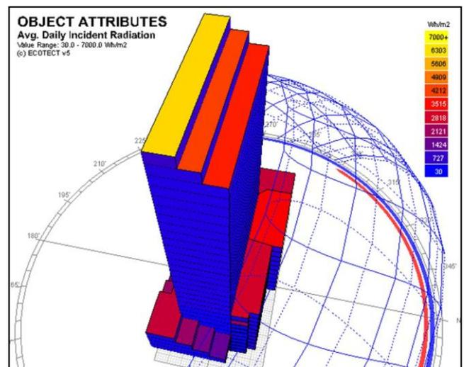
Total radiation absorption by the **NEW DOUBLE ENVELOPE OF THE BUILDING (2014)**. note the range is between 0.07 to 6 kwh/m<sup>2</sup>. Derived from: Autodesk Ecotect
