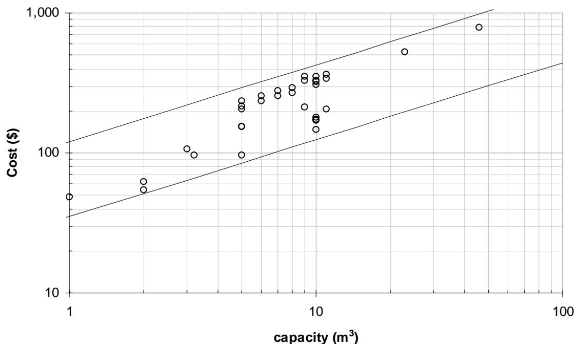
The costs follow a mathematically predictable rise, particularly when they are of a similar design. A cost estimate of a tank of any required size can therefore be made from cost data of another sized tank by using the relation:
