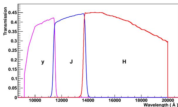
**Fig. 4.** Overall transmission of the 3 bands of the Euclid NIR imaging system, in its current design. The H filter red cutoff has been pushed to 2  $\mu\text{m}$  compared to earlier designs. The cut-on of the y filter is determined by the dichroic that splits the beam between visible and NIR instruments.
