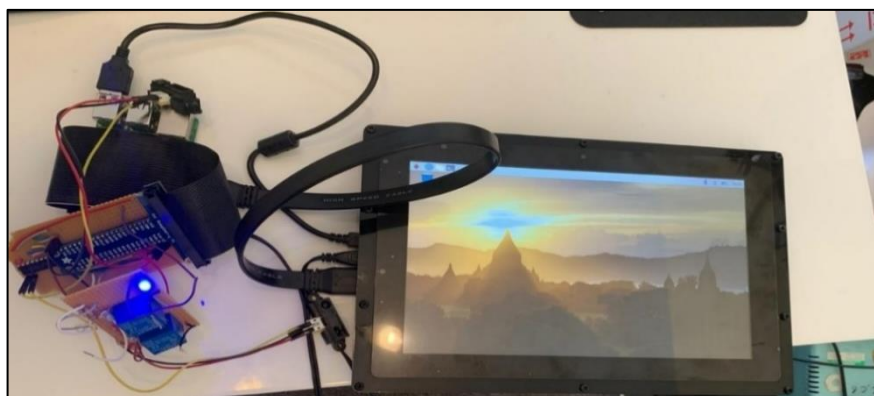
Fig. 8. Prototype of the new system showing a touch screen to input user settings.
