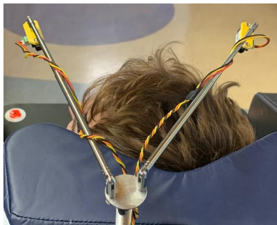
Fig. 5. IR sensors used to operate a powered wheelchair.
