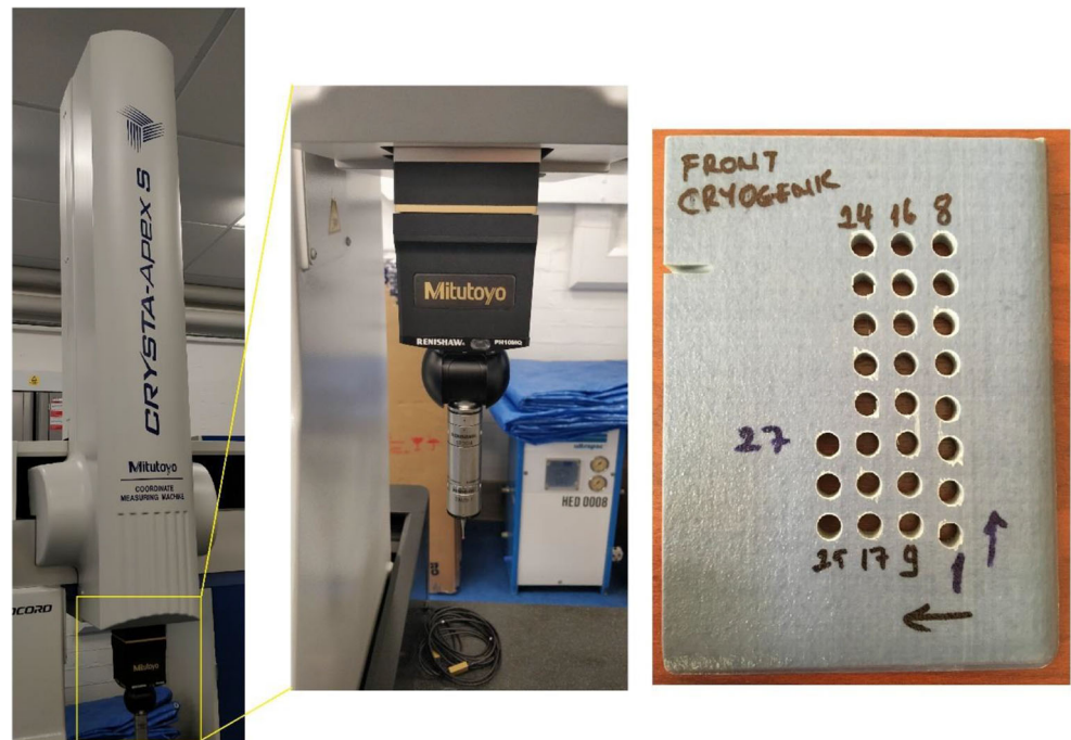
Fig. 2 Hole metrics measurement using CMM machine
