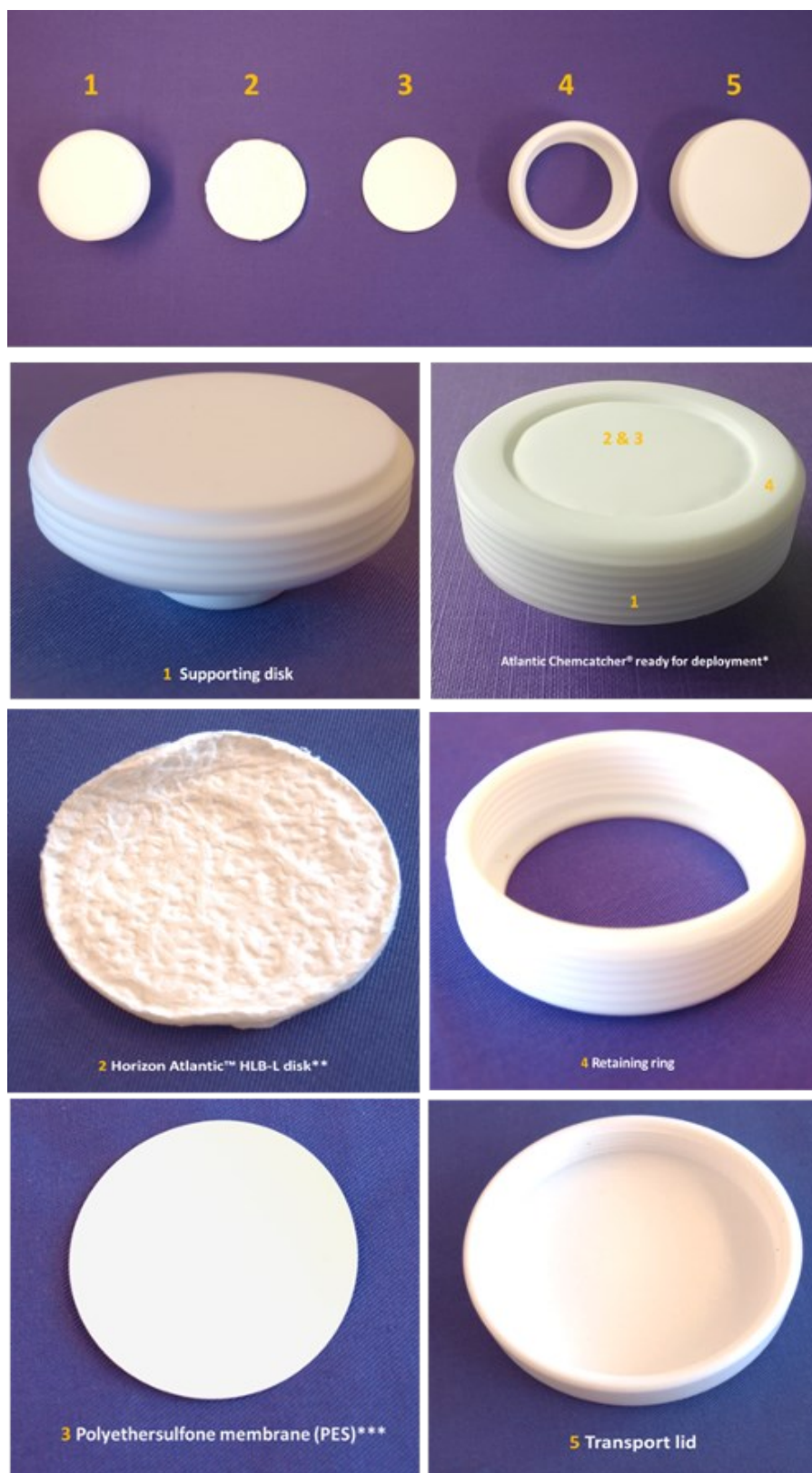
Fig. S1 Components of the Atlantic® version of the Chemcatcher® PSD. *The Chemcatcher® is made of machined PTFE, **Atlantic® HLB-L disk (47 mm diameter) and ***PES, Supor®200, pore size: 0.2 µm, 52 mm diameter disk.
