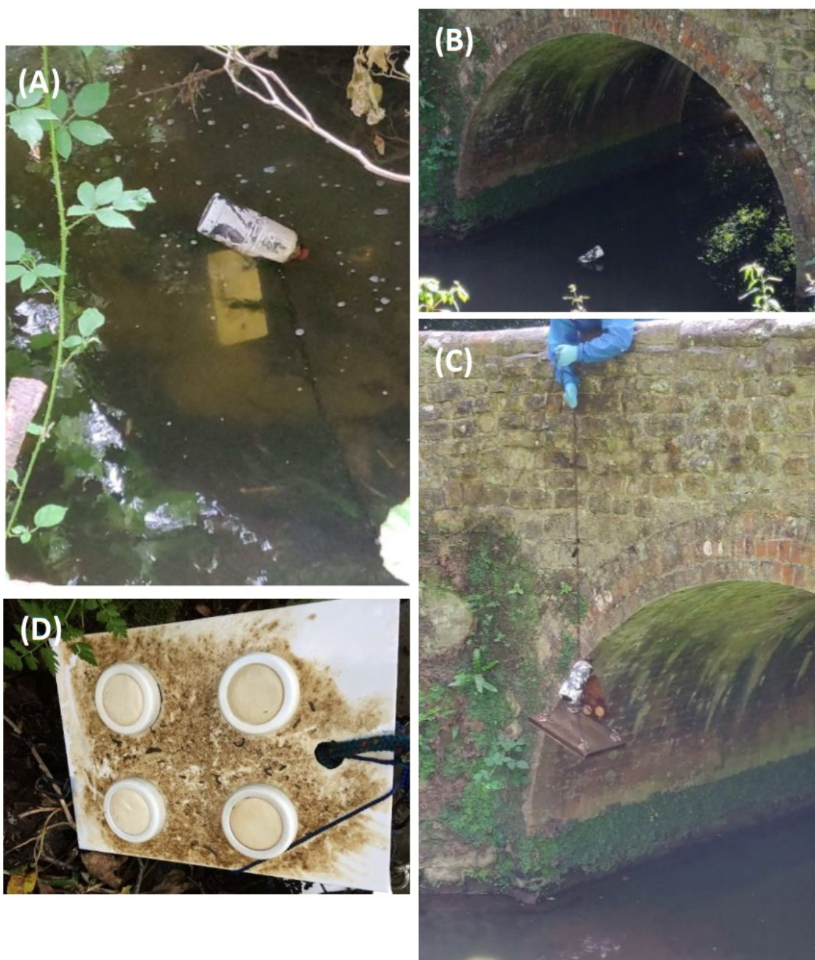
Fig. S3 Photographs of a rig type deployment system, showing Chemcatcher® devices during deployment (A), (B), during retrieval (C), and 4 Chemcatcher® devices secured in a plastic mount after retrieval (D).
