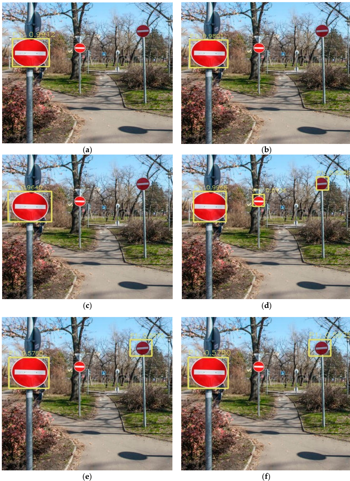
Figure 6. Recognition test for prohibitory sign class P1 by (a) Yolo V3 1, (b) Yolo V3 2, (c) Yolo V3 3, (d) Yolo V3 SPP 1, (e) Yolo V3 SPP 2, and (f) Yolo V3 SPP 3.
