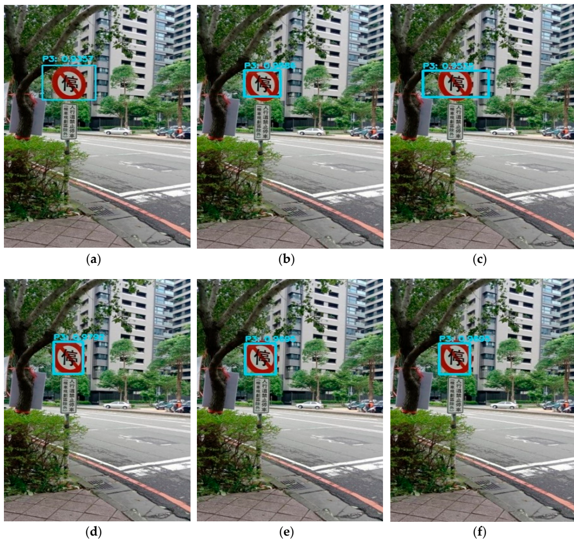
Figure 5. Recognition test for prohibitory sign class P3 by (a) Yolo V3 1, (b) Yolo V3 2, (c) Yolo V3 3, (d) Yolo V3 SPP 1, (e) Yolo V3 SPP 2, and (f) Yolo V3 SPP 3.
