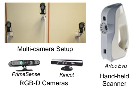
Fig. 7. Multi-camera setup [55], RGB-D cameras [57], [58] and 3D hand-held scanner [60] used in 3D facial motion capture systems.
