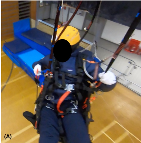
Figure 7. (A) Participant attempts to extract deployment bag using an upwards pull, causing the bag to stick. (B) Rather than adjust the angle of pull more laterally, the participant changes their grip so they can pull upwards with more force.
