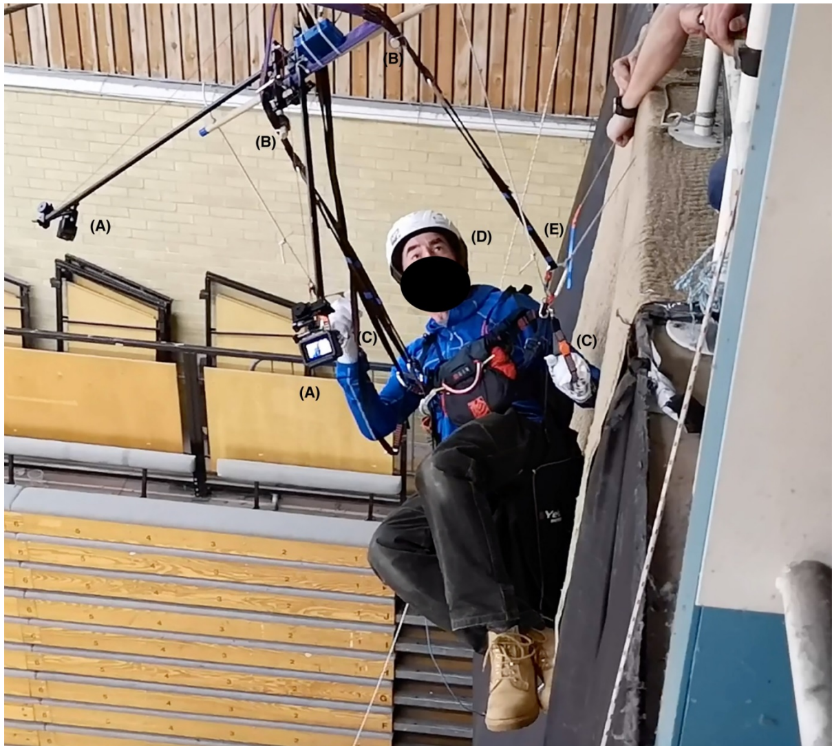
Figure 2. Zipline set up in the moments before release for a participant with a front-mounted system. (A) Cameras; (B) LED lights; (C) Hands in control lines responding to the light sequence; (D) Gaze directed upwards; (E) Tensioned release.
