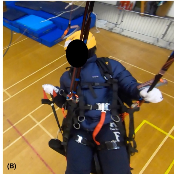
Figure 7. (A) Participant attempts to extract deployment bag using an upwards pull, causing the bag to stick. (B) Rather than adjust the angle of pull more laterally, the participant changes their grip so they can pull upwards with more force.
