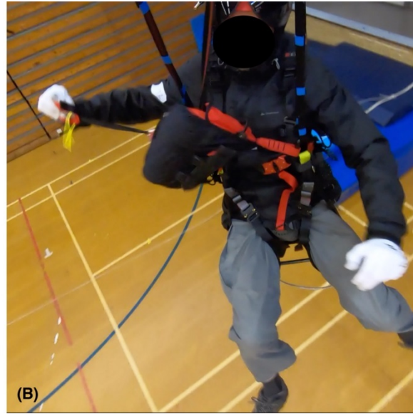
Figure 11. (A) The participant easily grasps the reserve handle of his front-mounted system. (B) As it was unsecured at the base, the container lifts up before the deployment bag is extracted, increasing difficulty of extraction and reducing the mechanical advantage of the subsequent throw.
