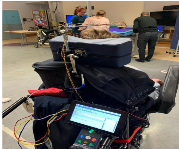
Fig. 5. Modified New system interfacing to IR head switches.
