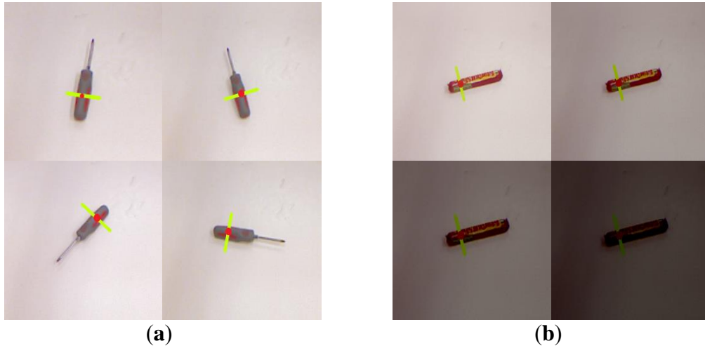
Figure 6. Grasp pose detection results under artificially changed environment: (a) The grasp pose detection results of the object with different poses; (b) The grasp pose detection results influenced by illumination.
