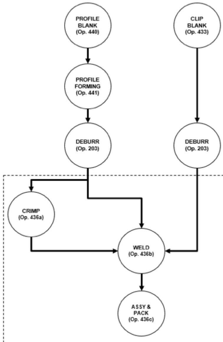
Figure 7: The VPP 096 Clamps processing flow diagram
