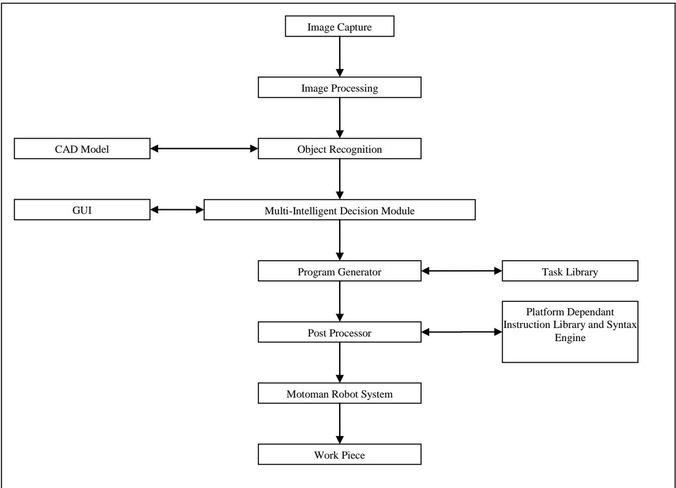
Figure 4 – Proposed System Flow Diagram
