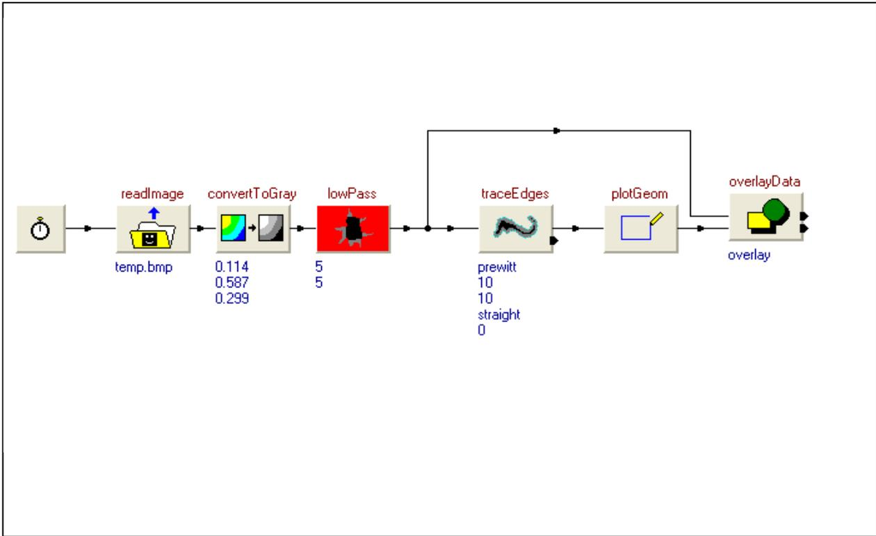
**Figure 8 – Visual Representation of Edge Detection Algorithm**
