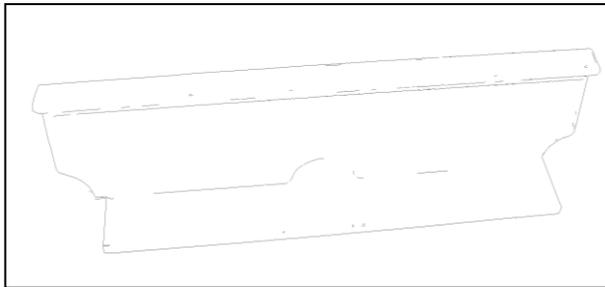
**Figure 11 – Image output from Edge Detection Algorithm**
