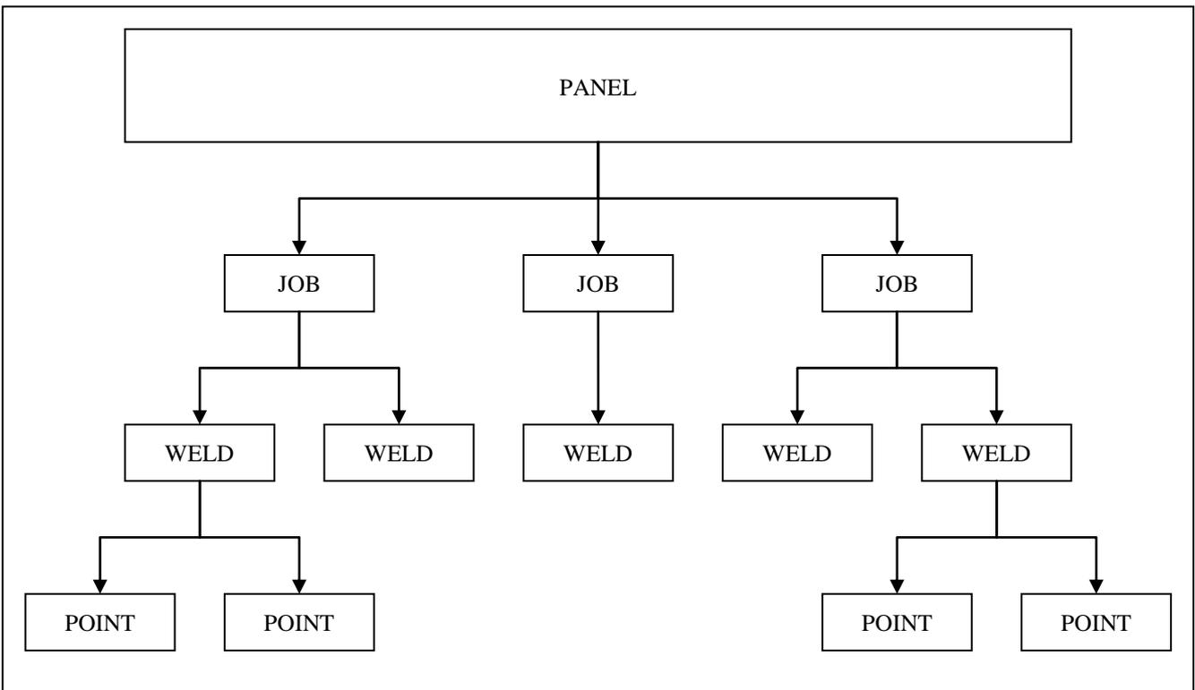
Figure 5 – Hierarchy of a Ship Panel
