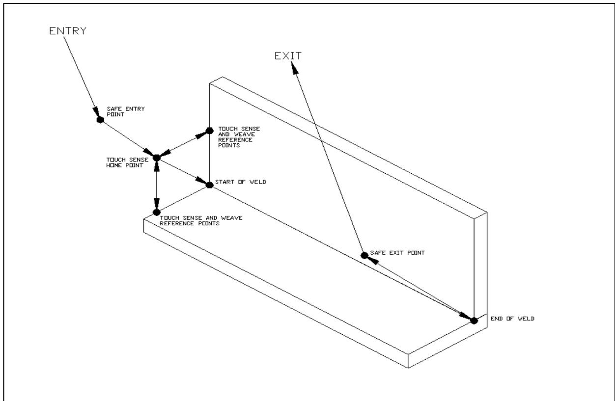
Figure 7 – End Effector Path Diagram
