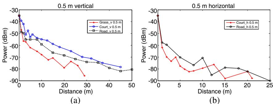
**Figure 5.** Comparison of signal variation at the same height over different surfaces for (a) vertical and (b) horizontal antenna orientations.
