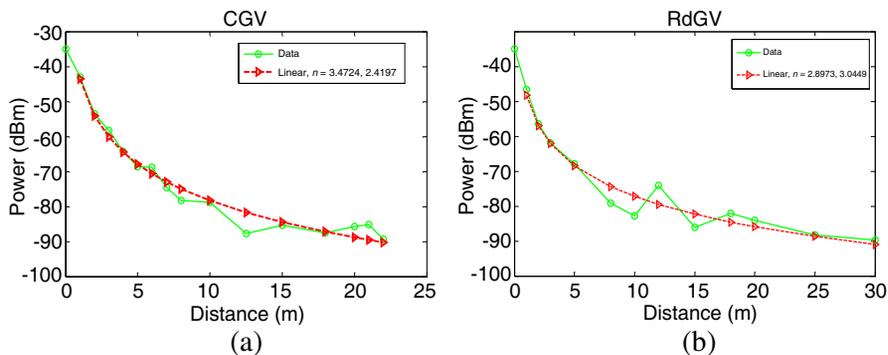
**Figure 7.** Model fitting to large scale signal variations for ground level antenna height on (a) sport court and (b) road.
