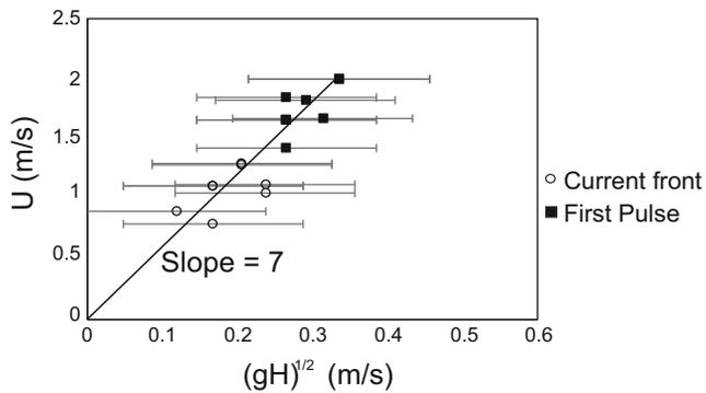
**Fig. 5** Froude number for the fronts and first pulses of selected experimental currents. Uncertainties in velocity are smaller than the size of the symbols. Uncertainties in current height are relatively large due to the thinness of the current fronts relative to video resolution
