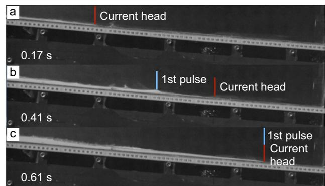
**Fig. 4** High-speed video frames of an experimental current on a 4° slope under  $0.93-0-0 U_{mf\_st}$  conditions (Fig. 2). Numbers on left are time in seconds since the current front entered the frame. **a** The front of the current enters the frame. **b** The current front continues to run out as the first pulse catches and begins to override it. **c** The current front is completely overtaken by the first pulse. A video of this experiment is presented in Online Resource 1
