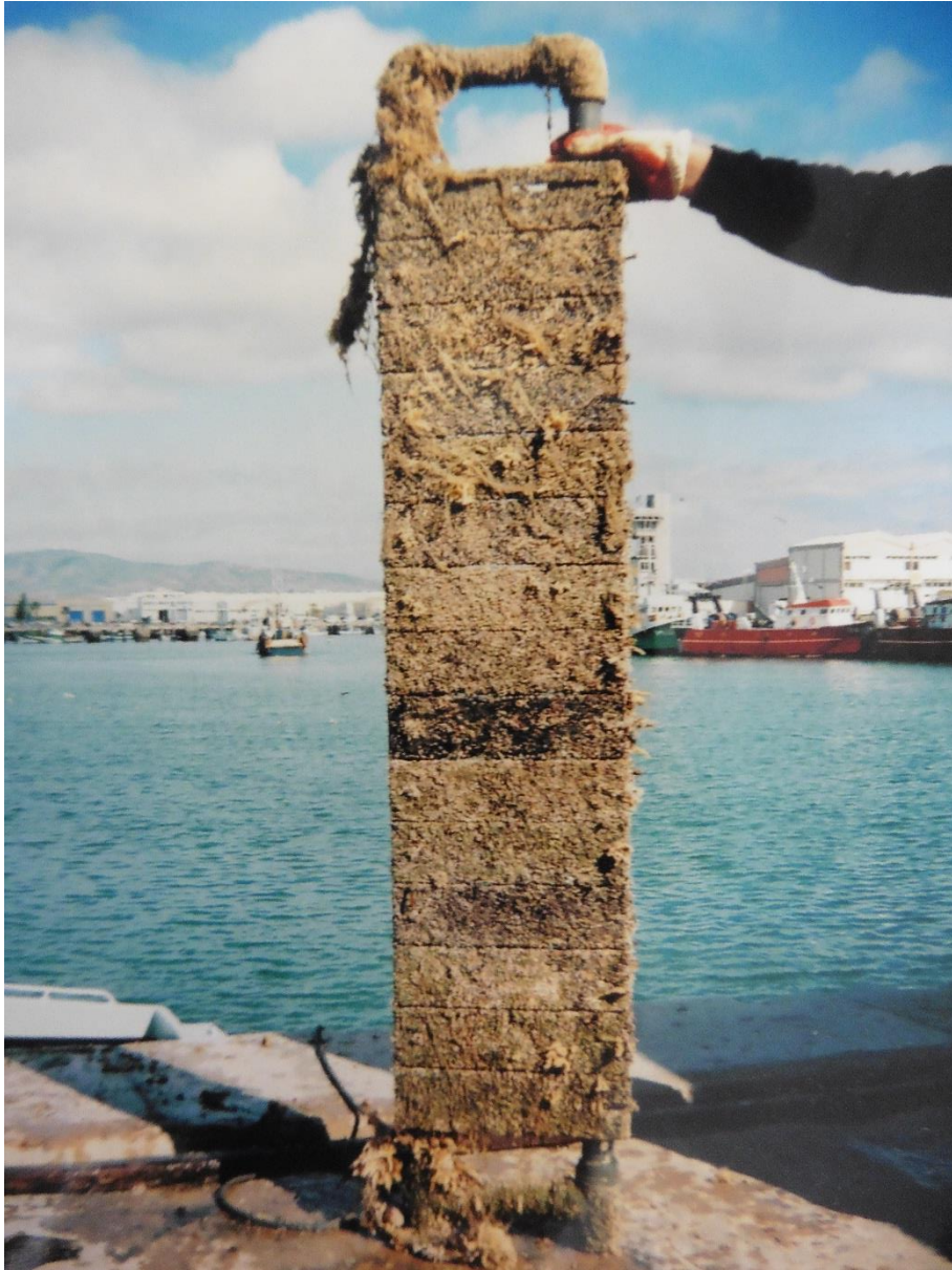
Figure 9: Typical marine fouling on a number of test racks after six months immersion.
