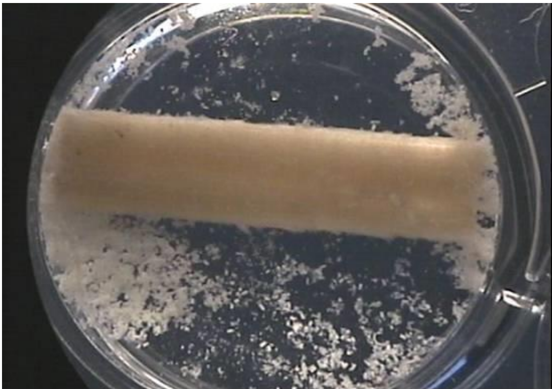
Figure 6: High feeding rate observed in a chamber containing a stick of European redwood sapwood which confirmed the vigour of the limnoriid population.
