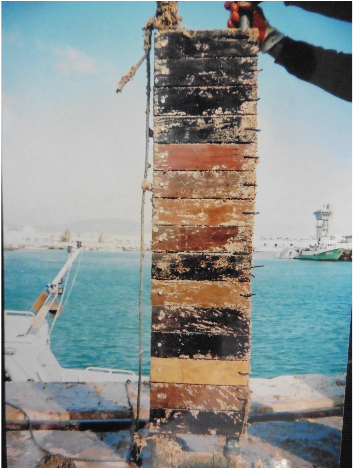
Figure 10: General appearance of test racks after cleaning to facilitate X ray photography.
