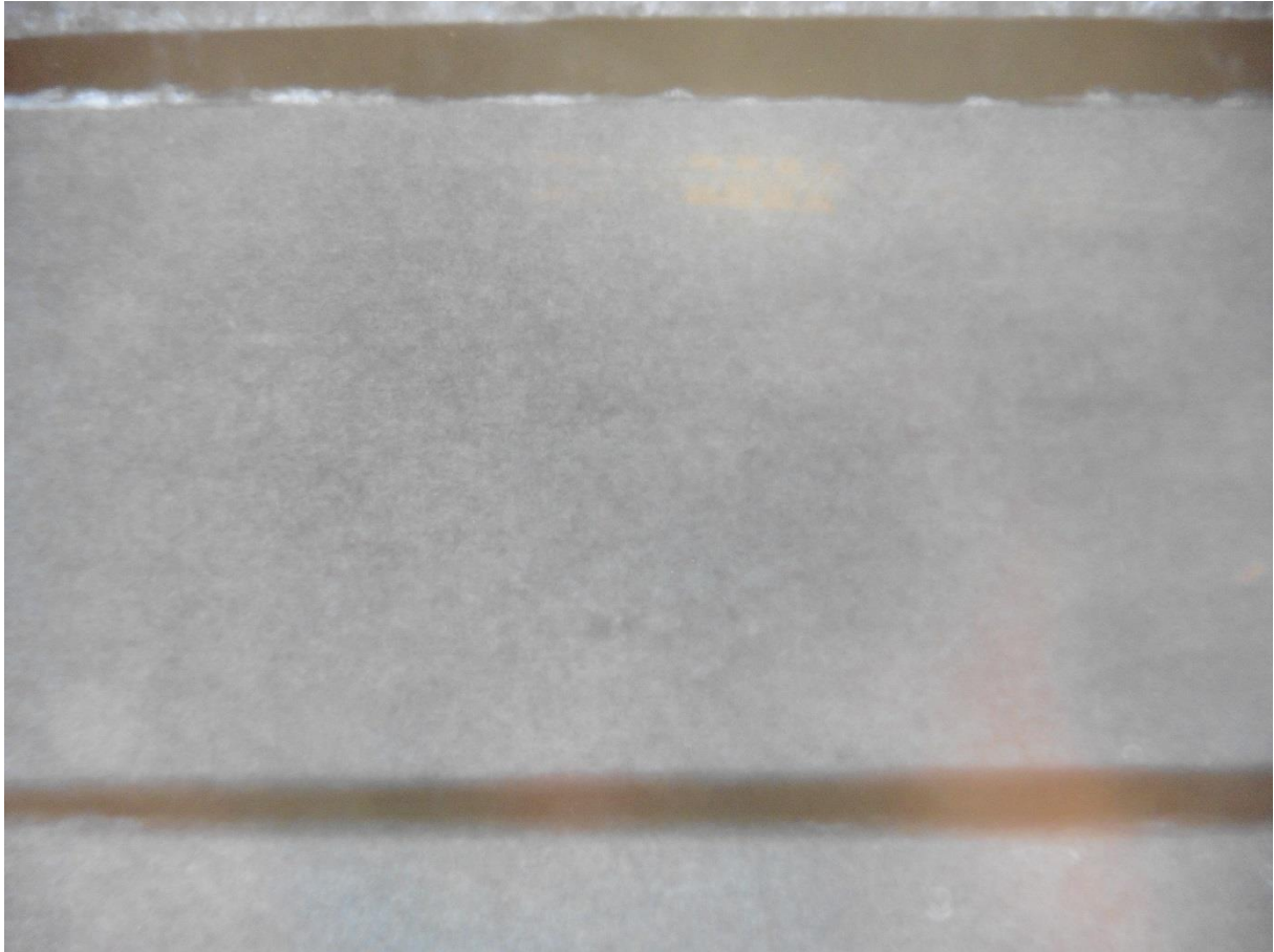
Figure 15: No evidence of teredinid attack in a specimen of the LUS angelim vermelho.
