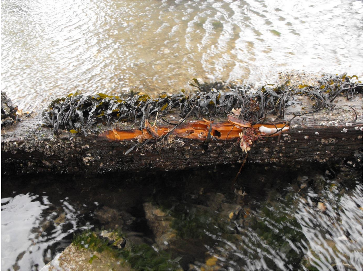
Figure 4: Example of the typical damage caused by teredinids
