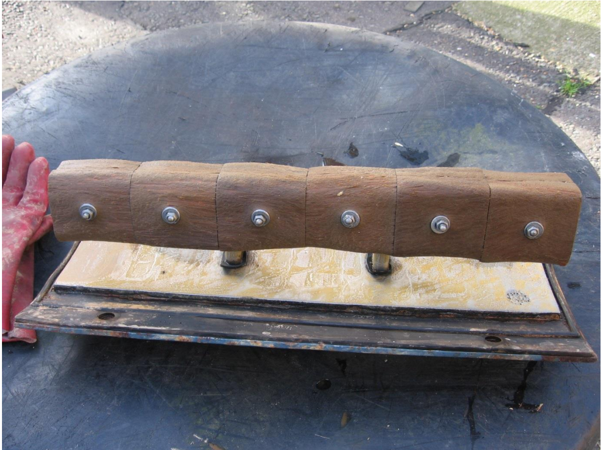
Figure 8: A test frame holding eroded greenheart test blocks after 160,000 revolutions.
