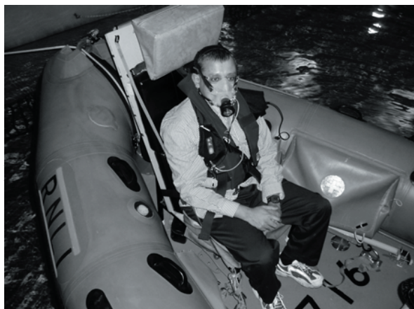
Fig 1. A subject secured into the HES seat on the bow of the Atlantic 75 lifeboat ready to begin the experiment.
