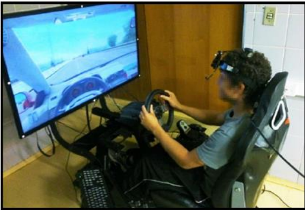
Figure 1. Participant on cockpit driving on the simulator and wearing Head-mounted Eye Tracker (ASL, H6).
