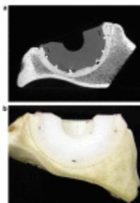
Debonding at the bone–cement interface of a sample tested under descending stairs loading condition. (a) A CT scan image showing clear demarcation at the bone–cement interface; (b) almost complete separation of the bone–cement (more ...)
